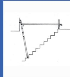
Insert adjustable legs into corner of platform to set to correct level and working height.
