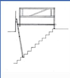
In wider or larger stairwells fix the optional guardrail frame into position to prevent falls.
