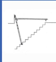
Place one end of platform onto the ladder frame with opposite end spanning to top of the stairs.
