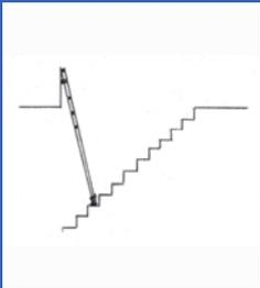
Position ladder frame on stairs at a suitable incline against the wall
