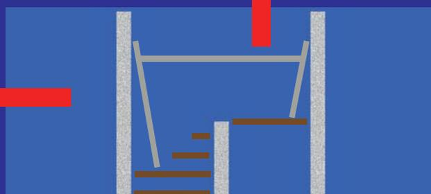
Section through stairwell showing frames and platform
